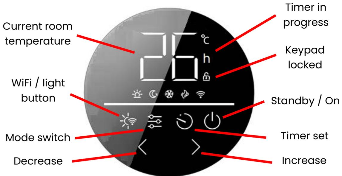
Figure 5: Control Screen Layout and symbols
