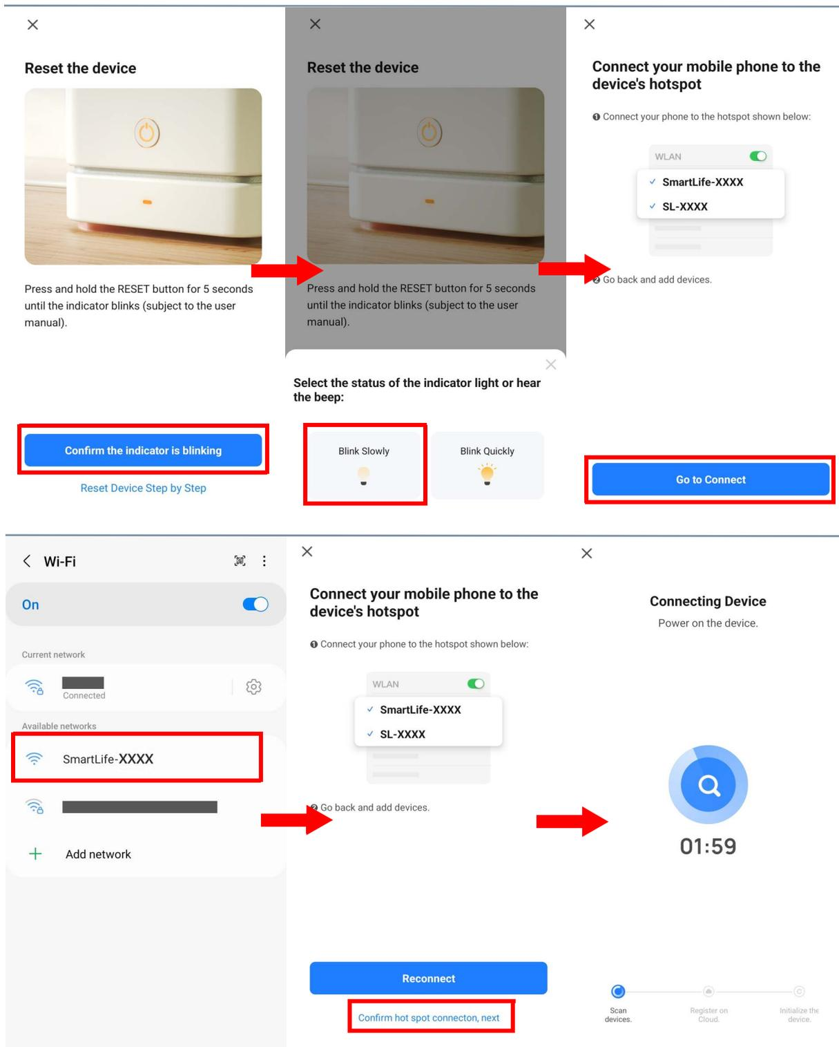
Figure 7: Connecting the heater to the app using AP Mode
